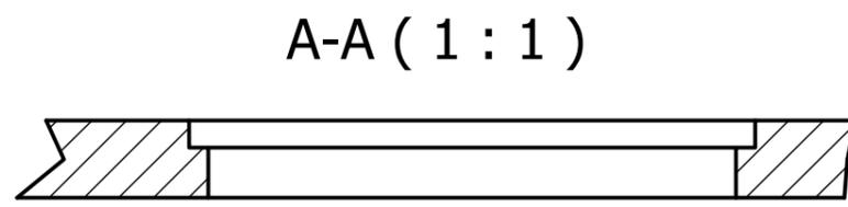
IN CASE OF MILLING THE PANEL INTO THE TABLE, MILL THE DRAWED CONTOUR TO A DEPTH OF 3.4 mm
